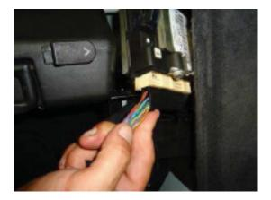
1. Remove the door cover located on the left side of the cargo area to expose the vehicles air suspension wiring harness and control module.
