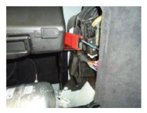
7. Connect the new plug to the electronic bypass module and secure it in a suitable location.
