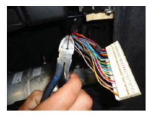
5. eparate the located wires and cut, leaving a suitable length to work with.
