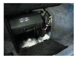
2. Remove both plugs located on the control module.
