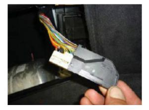
3. Remove the cover of the larger plug by sliding it off of the end.
