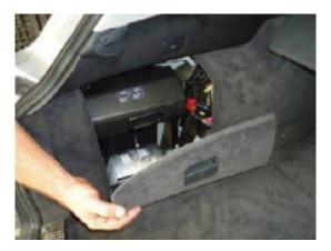
9. Do NOT plug wiring harness back into the vehicles air suspension control module. Replace the door cover.
