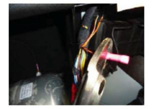
6. Strip the ends of the wires. Using the supplied butt connectors, crimp the electronic bypass module to the vehicle side of the wiring harness.
